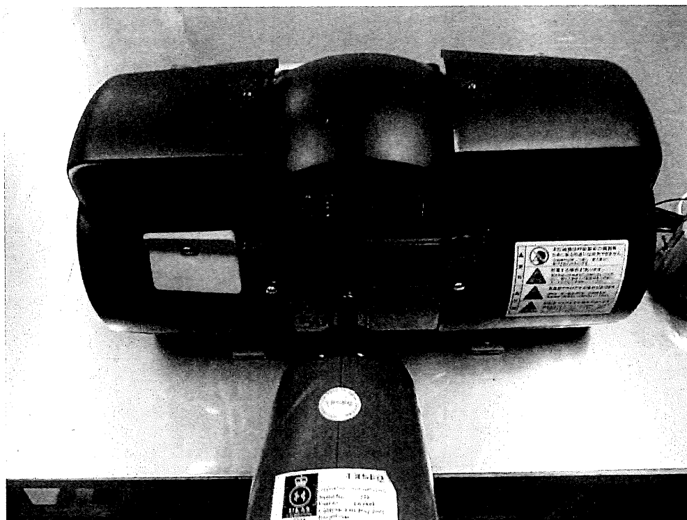
Photograph 16: Set-up for Electrostatic Discharges, Air Discharges
