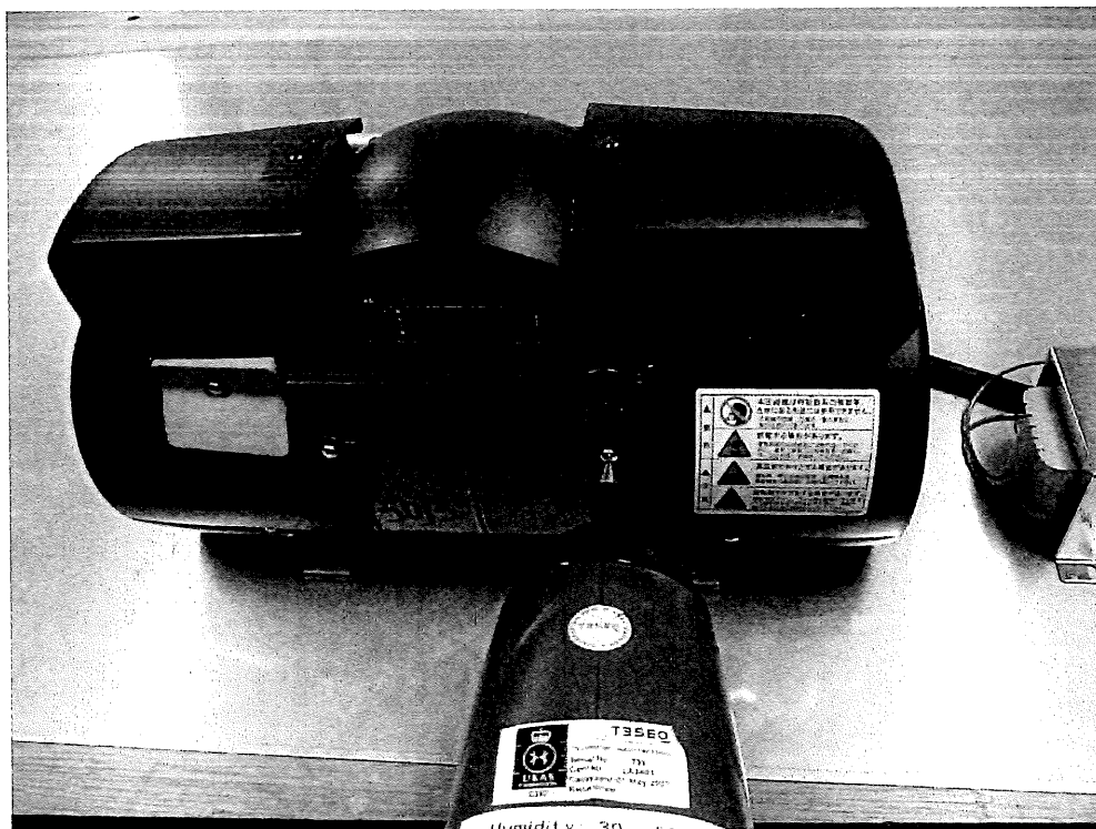
Photograph 15: Set-up for Electrostatic Discharges, Contact Discharges
