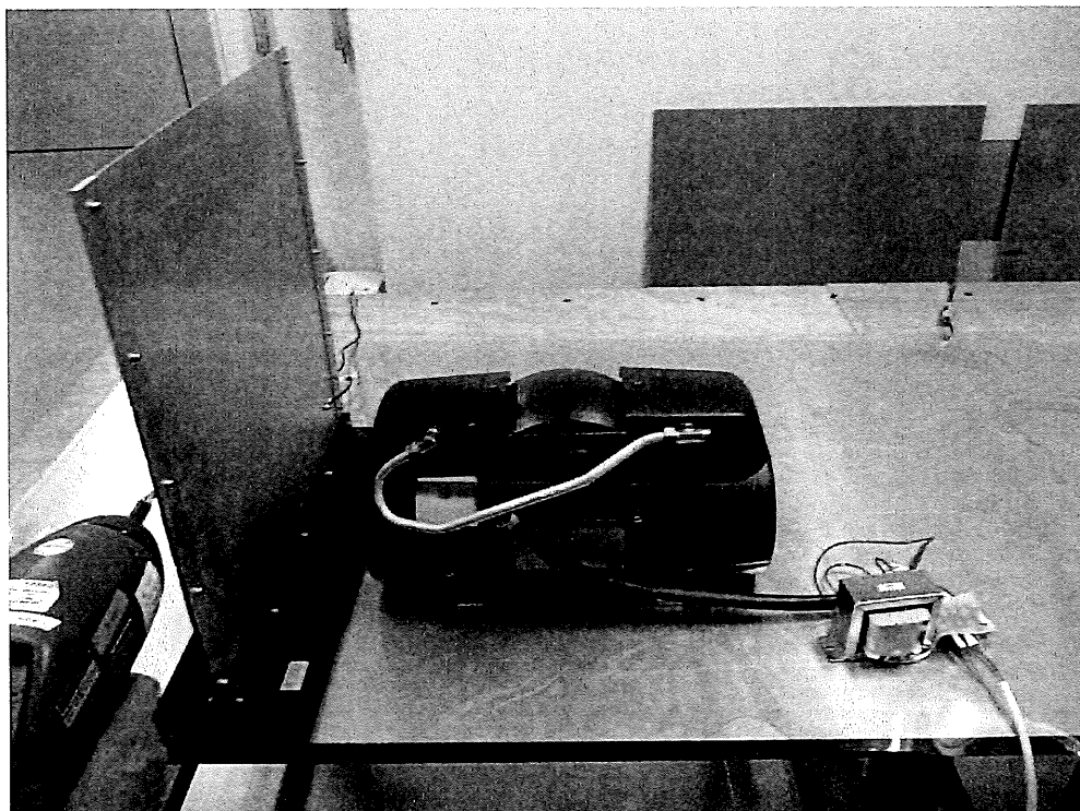
Photograph 14: Set-up for Electrostatic Discharges, VCP
